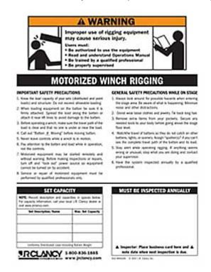
JR Clancy Rigging Instructional Sign for a Motorized Winch
