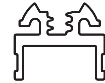
Single Beam Cap Profile suitable to use with a 2' x 2' (38 x 38) wood board.
