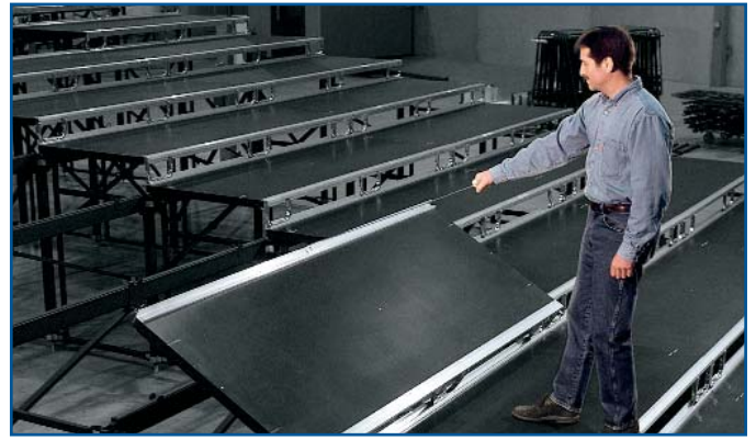
After the base structure is assembled, decks are set into position with a convenient lowering tool that eliminates back strain while facilitating placement.
