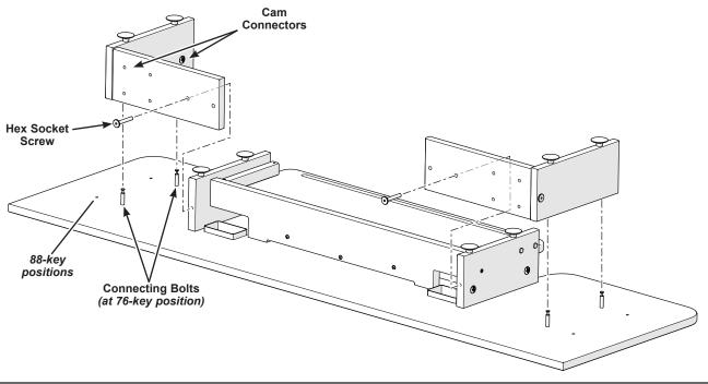
Set the workstation desk to fit on top of the piano as shown.
