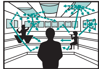
ACOUSTICALLY BALANCED ROOM WITH ABSORBER AND DIFFUSER PANELS Loudness is controlled. Performers can hear themselves and each other. Conductor has accurate impression of balance.
