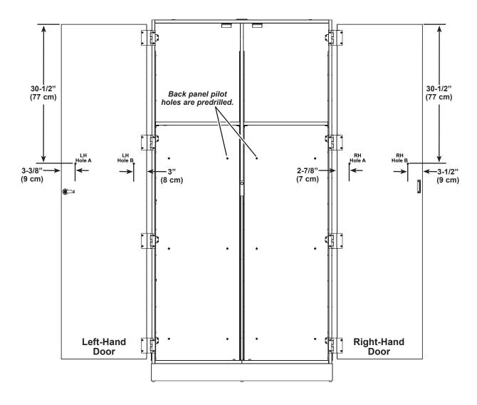
2. Using a 1/8" drill bit, drill pilot holes no greater than 1/8" (3 mm) into the door laminate surface at these two locations.
