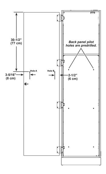
2. Using a 1/8" drill bit, drill pilot holes no greater than 1/8" (3 mm) into the door laminate surface at these two locations.
