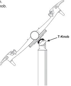
2. Loosen the side knobs to release the adjustable mount arms. Squeeze open the clamp on the lower arm and insert the tablet.
