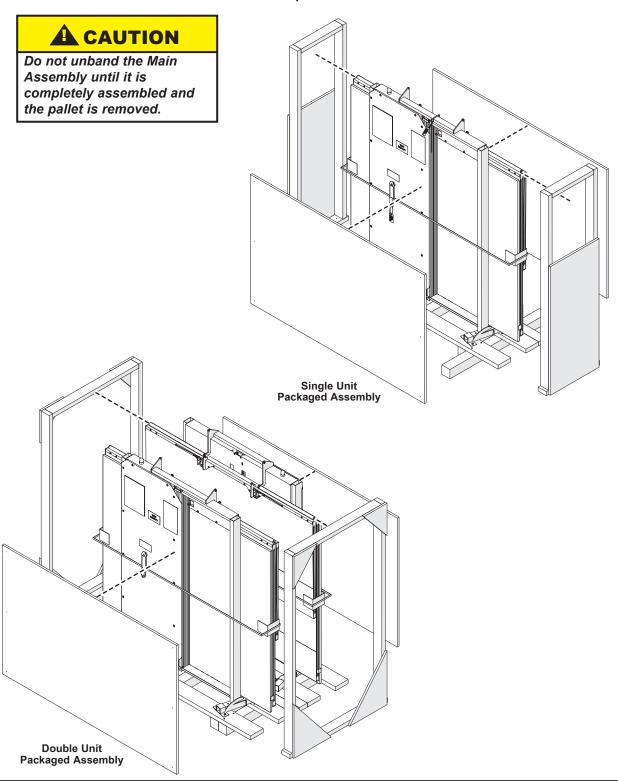
2. Remove the outer-most 4 x 4's from both sides.
