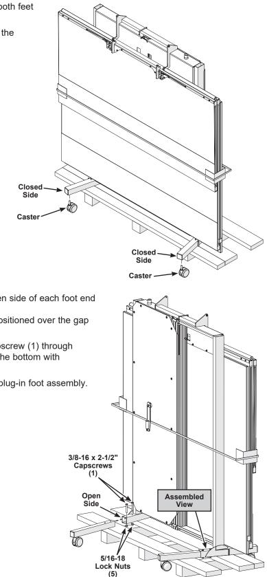
Slide one plug-in foot assembly into the open side of each foot end and align both sets of pre-drilled holes.
