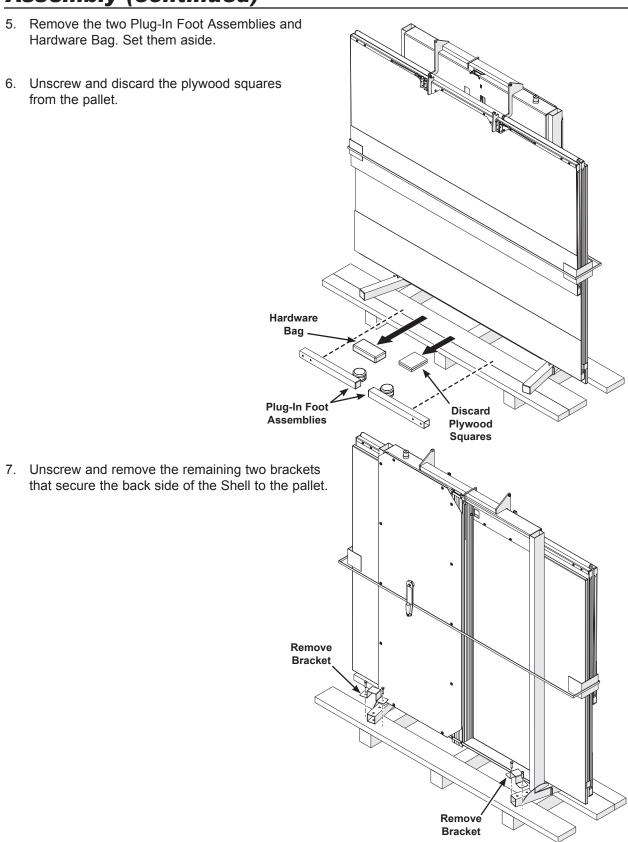
8. Slide the shell over until the closed side of both feet extend beyond the edge of the pallet.
