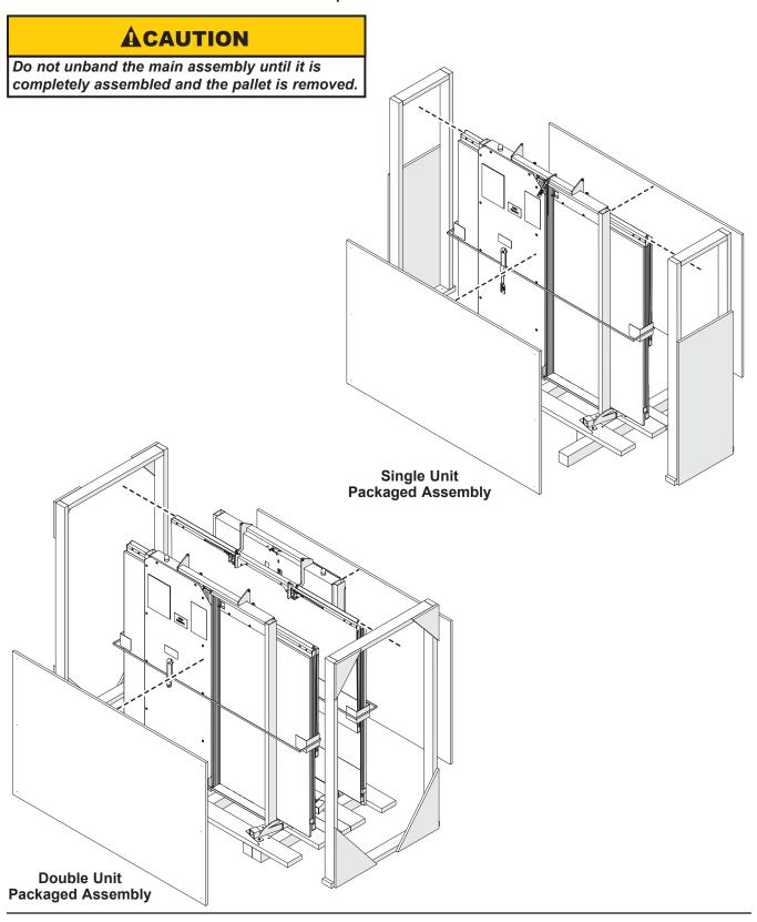
2. Remove the outer-most 4 x 4's from both sides.
