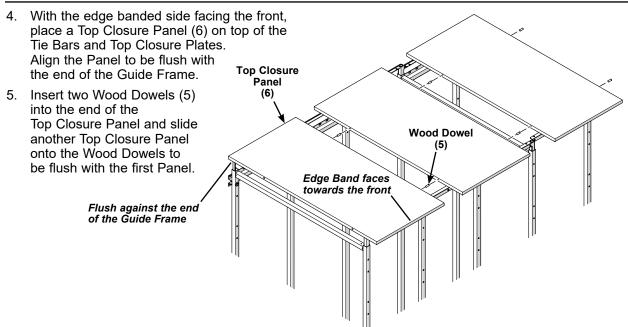
6. Continue adding on Wood Dowels and Top Closure Panels along the entire Guide Frame Assembly until the last full Panel fits on the top.
