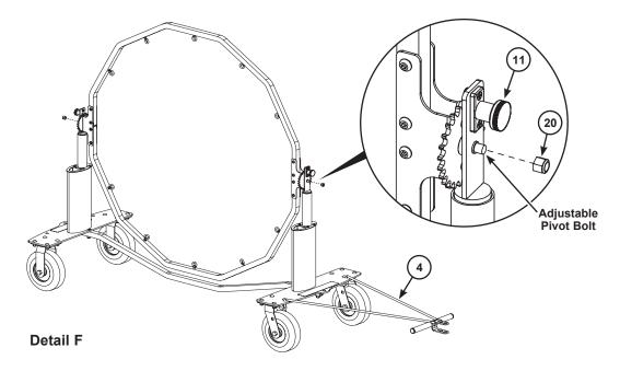
21. A separate tow bar (4) is provided which inserts into two holes in the cart base assembly (1). The tow bar may be used as a handle to pull the cart manually or can be attached horizontally to a lawn and garden tractor.
