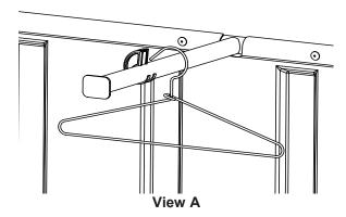
2. Locate hanger over bar into holder as shown in View B and rotate holder down so that the hanger is secure.
