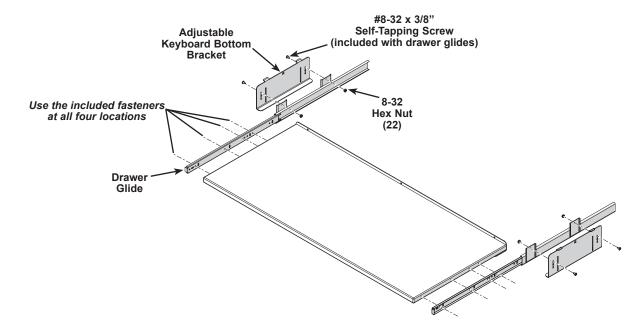
24. Fit the back of both drawer glides into the slots of the front wiring panel.
