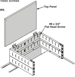
8. Close the top panel and secure it to the top rackmount shelf using two #10-32 x 1.25" pan head screws.
