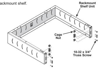
2. Attach the rackmount shelf to the desktop using six #8 x 5/8" truss head screws.
