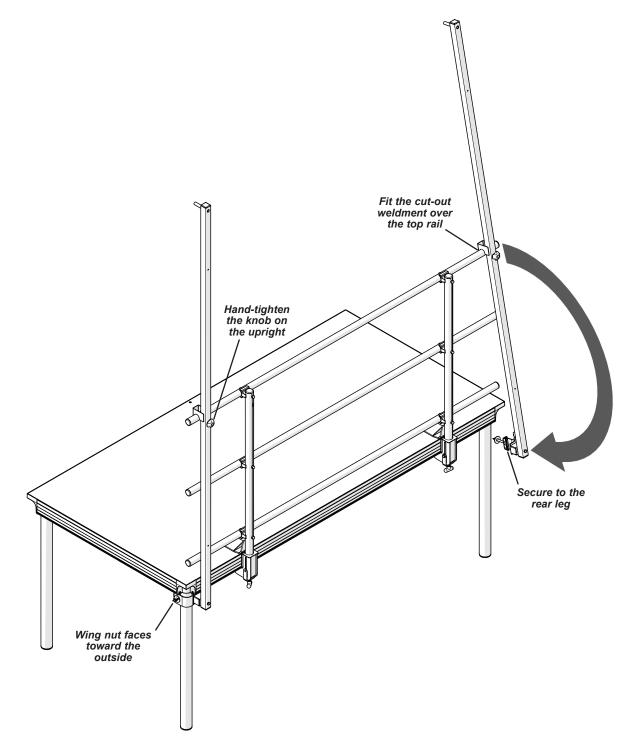
4. With the hook and loop surface facing the platform deck side, attach the horizontal bar to the top of both uprights using two 3/8-16 x 5" capscrews and 3/8-16 wing nuts.
