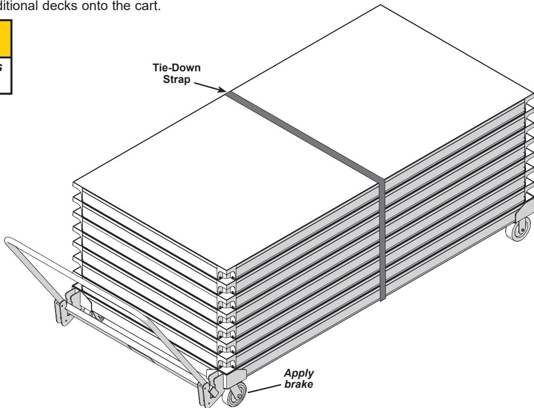
7. Secure the decks using the tie-down strap.
