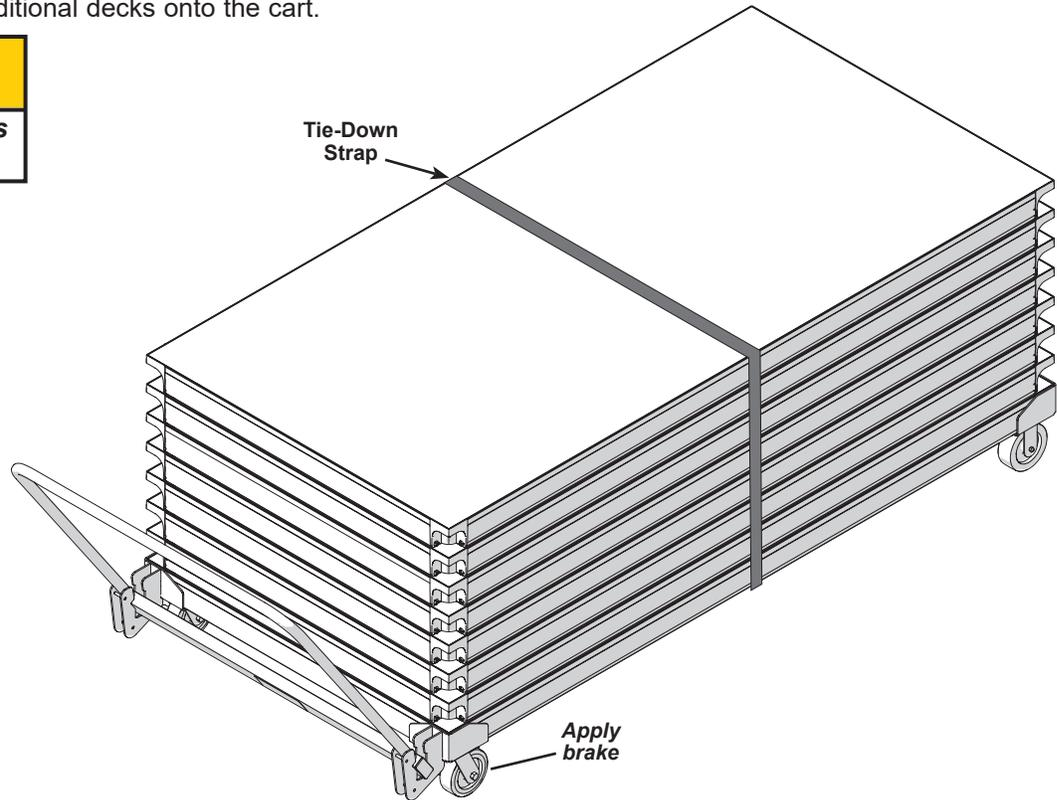
7. Secure the decks using the tie-down strap.
