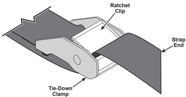
8. To release the strap, push on the ratchet clip and pull the strap loose.
