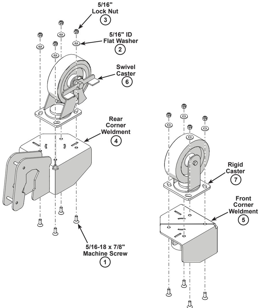
2. Attach each of the corner weldments to the underside of a StageTek rectangular deck.
