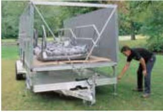
Easy, one-person setup in just minutes. Folding design uses gas-assist springs to provide smooth and safe operation. Built-in leveling jacks offer fast leveling on any surface.
