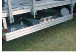
Space beneath stage deck for hauling equipment and cargo, with optional closure panels for increased security and weather-resistance.
