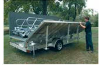
Stage folds down and has adjustable legs attached for solid deck support.
