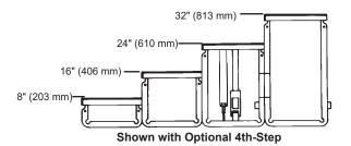
4'  $\times$  18" (1219  $\times$  457 mm) Riser = 65-1/4" (1657 mm) long  $\times$  20.6" (523 mm) wide 4' 7"  $\times$  24" (1397  $\times$  610 mm) Riser = 67" (1702 mm) long  $\times$  26.8" (681 mm) wide 6'  $\times$  18" (1829  $\times$  457 mm) Riser = 83-1/4" (2115 mm) long  $\times$  20.5" (521 mm) wide Optional 4th-Step must be removed prior to folding for storage
