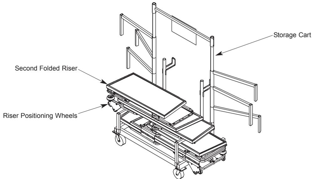
6. Close the two Swing Arms above the Riser. It will be necessary to lift all of the Arms high enough for the two Arms to clear the Riser.
