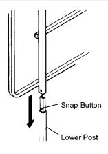
With standard step arrangement, rail loop and cross brace should be in *front* of posts. With reversed steps, they should be *behind* posts.
