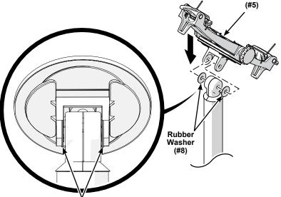
Rubber Washers fit between the Tablet Mount and Pivot Hub
