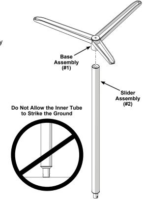
Attach the Base Assembly to the Slider Assembly using a 1/4-20 x 1.25" Socket Screw (#3).
