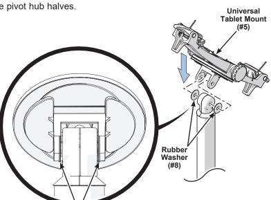
Rubber Washers fit between the Tablet Mount and Pivot Hub **Pivot Hub**
