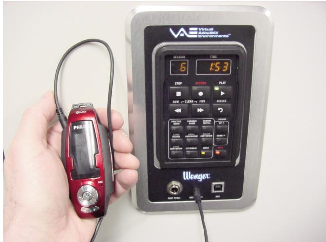
*Be sure the VAE system is muted by pressing the MUTE button on the control panel. This will turn off the VAE microphones in the room so indirect noises are not recorded and minimizing accidental "doubling" of the VAE acoustic effects.*
