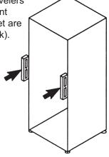
2. Adjust the levelers on one side until the front edges of the cabinet side panels are plumb (side-to-side).
