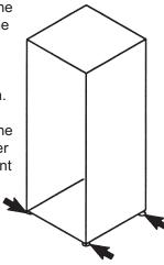
Adjust both front levelers equally until the front edges of the cabinet are plumb (front-to-back).
