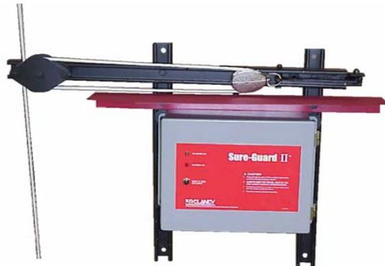
To ensure proper operation, the tension in the release line must be set between 5 & 40 pounds (3 & 18 Kg). See the fire safety curtain system drawings for additional details on installing the release line and rigging for your specific system.
