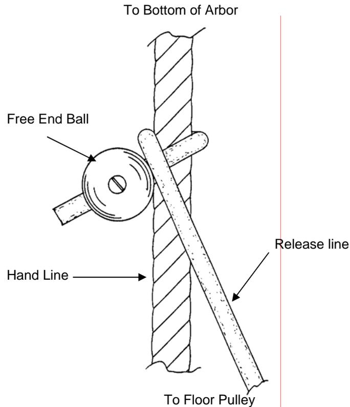
This type of system requires some practice and angle at which the release line is attached to the handline is critical. Too little of an angle, and the curtain will not deploy. Too much of angle and the release line won't hold. Additional weight may be added to the release line either before or after the floor block to aid in the quick freeing of the line. If you are having difficulty with setting your release, contact a professional stage rigging company.
