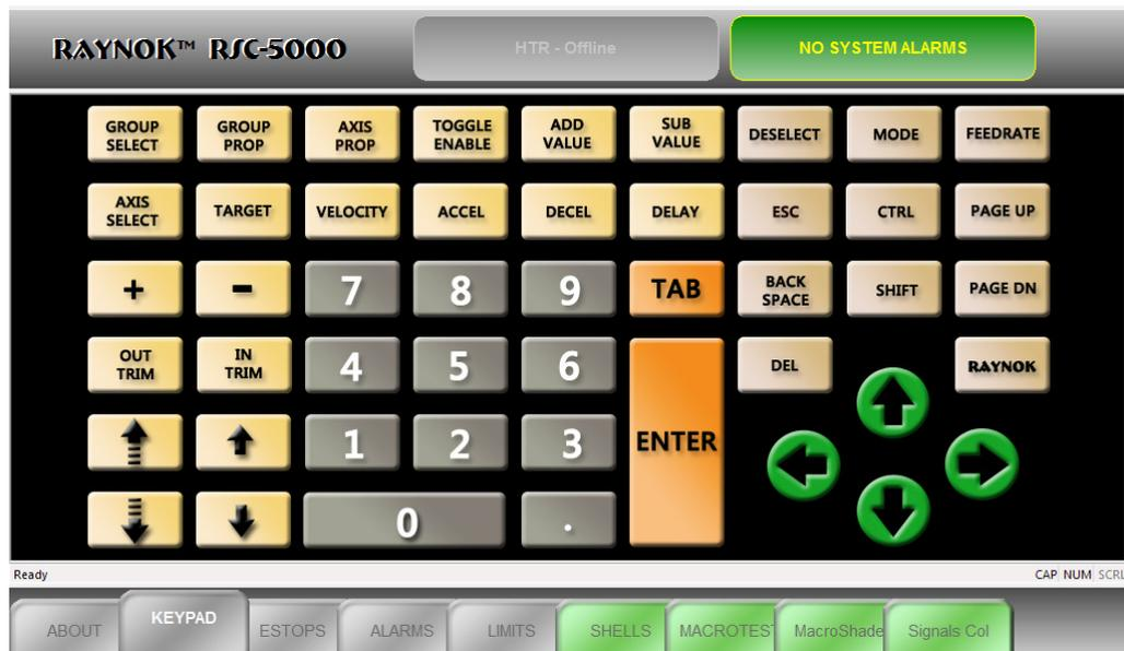
The KEYPAD Tab is a pre-configured macros button tab. This tab's layout has been created based on the macros that will be used most frequent to speed up the user's ability to command the system. This view is not configurable by the end user and is preparatory to the **RSC-5000 TOUCHSCREEN INTERFACE**.
