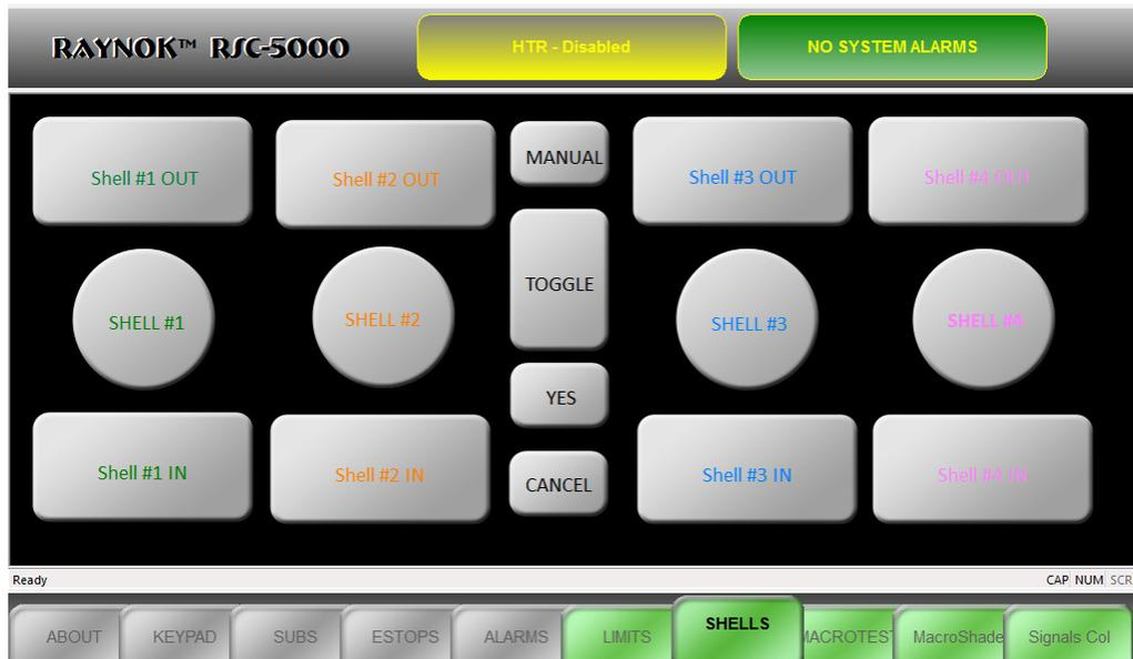
The **RAYNOK RJC-5000 SOFTWARE** is capable of displaying Signal and Macro views directly mirrored from the main **RAYNOK SOFTWARE**. The screenshot above is just one example of what can be done with this view. To add a Macro View Tab, add a new view within the main **RAYNOK SOFTWARE** in the 'Console Views' section of the 'Views' tab:
