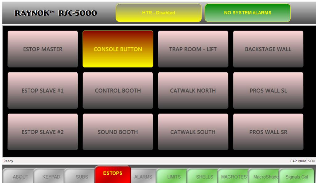
The E-STOPS Tab is a pre-configured console view tab used specifically to display the systems E-Stop reporting. This view uses a signal group named 'All Estops' to display its signals. To setup and/or edit the ESTOPS Tab view refer to the **RAYNOK SOFTWARE MANUAL** sections regarding Signal Groups and Macros Views.
