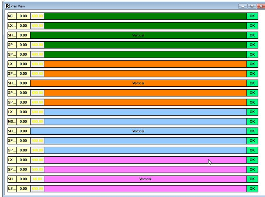
The *Plan View* is a good way of monitoring cues and controlling axes. This simple and informative layout is set up so that everything can be done effectively in a single space, without having to switch to different views. Each bar created represents an axis, partitioned into several blocks displaying axis condition, current position, and limit/interlock indicators. Different states of the axis are represented by simple word descriptions - such as “linked” or “disabled” - and colours.
