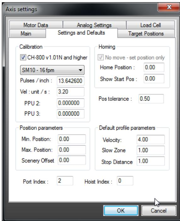
**Calibration:** Select the chain motor that is attached to the axis. Pulses/inch and Vel will automatically be readjusted according to the configuration chosen. Alternatively, the “other” option can be selected and the motors can be calibrated as any other axis.
