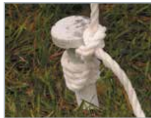
Ropes and ground anchors hold the shell firmly in place and can withstand winds up to 20 mph (32km/hr).
