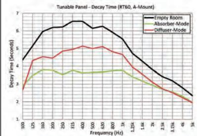
Provides up to .8 seconds of change in reverberation time. Test is actual independent lab test conducted by Riverbank Labs.
