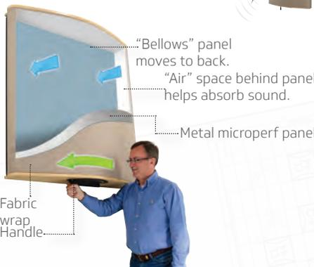
Sliding the handle to the left puts the panel in Absorption mode.
