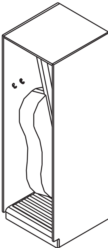
Bass and Cello Protective Kit installed into a #8 or #9 Instrument Storage Cabinet
