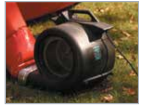
A blower motor operates quietly and inflates the shell in less than ten minutes.
