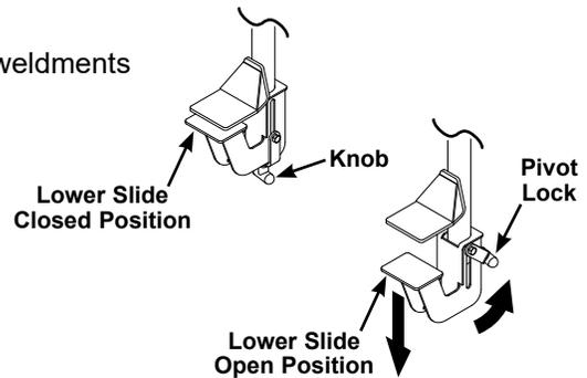
2. Using two people, lift the guardrail assembly to rest on the stage deck as shown. The lower slides should fit under the edge of the stage deck and be tight against the bottom of the stage deck when in the closed position.
