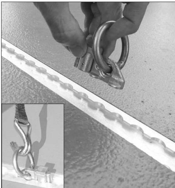
11. Unhook the tie-down straps from the tie-down loops (inset photo) and unload the railings and other stage hardware. Remove each tie-down loop from the channels in the stage floor: lift the round part and slide it along the channel until its flanges align with openings in the channel.
