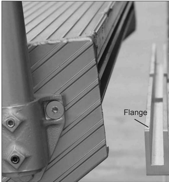
3. Slide the attachment flanges into place in the stage edge at the stair location. With a helper, position the stair assembly with the top edge of the top tread at the flanges. Lift the bottom end of the stair to slide the top edge onto the flanges, then lower the bottom end to secure the stair assembly in place.
