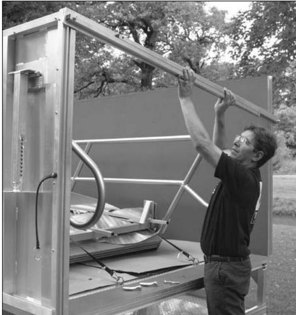
8. Remove the top brace assembly at each end. If a helper is available, have them help hold the decks upright, especially on a windy day.
