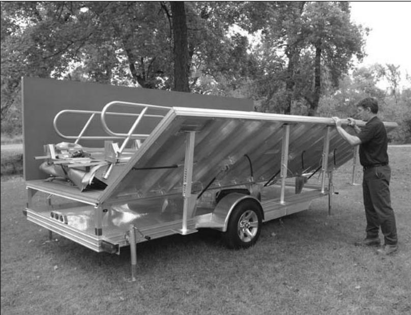
9. Begin lowering one stage deck. The deck supports will swing out as the deck is lowered. Lower the deck until the support feet rest on the ground.
