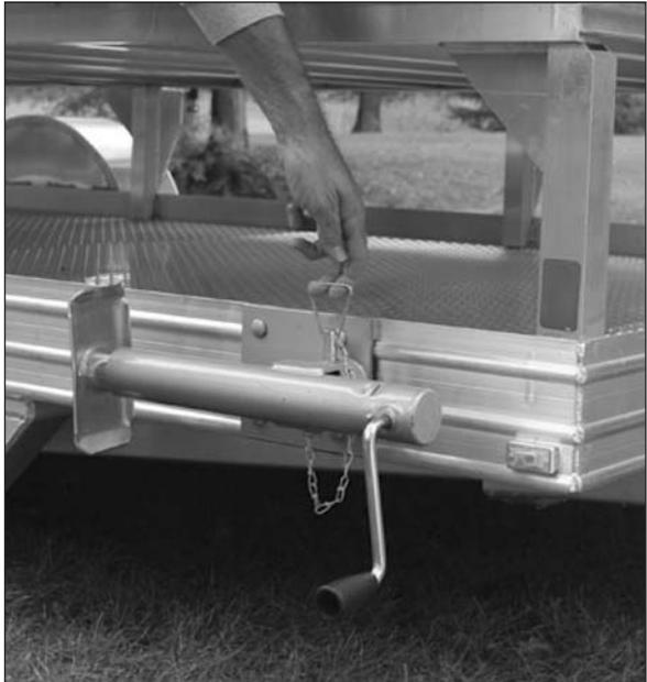
2. Pull the locking pin from each of the four manual leveling jacks located near the trailer corners. Rotate each jack from its traveling position so the foot of the jack faces the ground.
