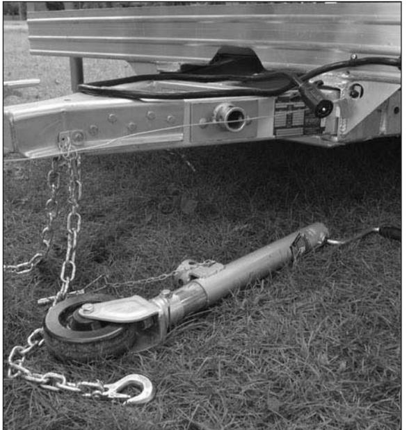
4. Raise the hitch jack wheel and remove the locking pin. Remove the parking wheel from the trailer hitch.
