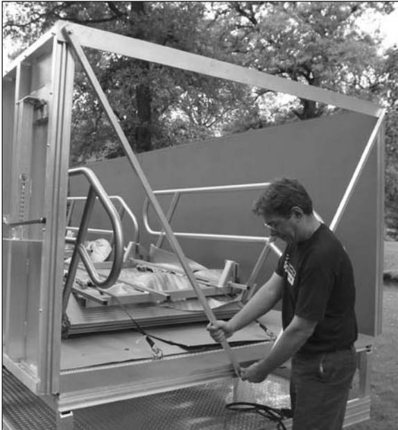
7. Unscrew the fasteners holding the traveling braces at each end of the trailer. Remove the diagonal braces from the fasteners.
