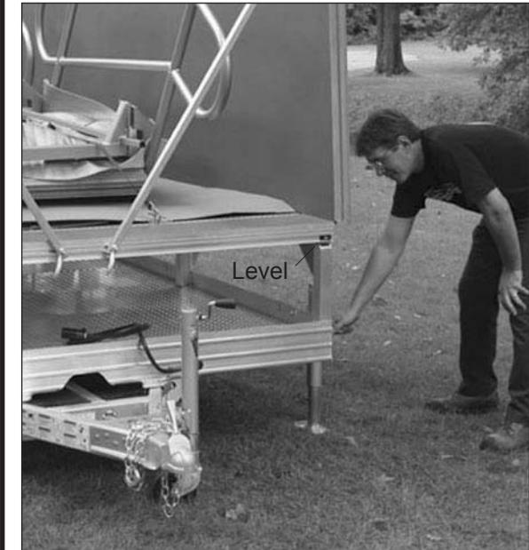
3. Turn the jack crank arms to bring each foot in contact with the ground. Use the small bubble levels located at opposite trailer corners and adjust the jacks until each foot is firmly against the ground and the trailer is level.
