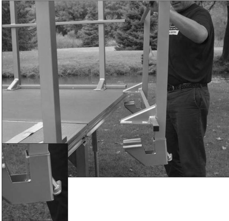
1. Lift each railing section into position, sliding the “C-clamp” feet over the edge of the stage. Note the position of the T-handle that will be used to tighten each foot once the railing is in place (see inset photo): each T-handle must be loose and resting on the outer edge of the railing frame for the feet to slide over the edge of the stage.
