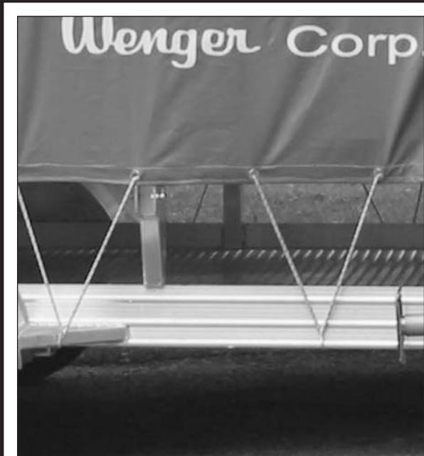
1. Unhook the tarp's elastic strap from the trailer frame and remove the tarp covering the trailer. Fold and store the tarp in the storage area under neath the trailer body.
