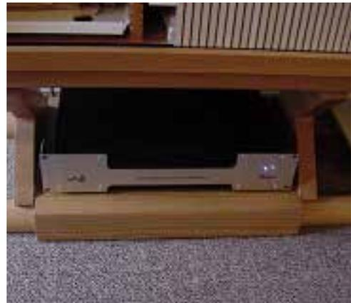
*If the installation will use the optional equipment rack, mount the processor in the rack before making any connections to the processor. The exterior of this optional rack may have items stacked around it on the top bottom or sides. The front and back should remain unobstructed for ventilation.*
