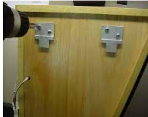
4. Press the female half of the loudspeaker grill guides into each of the eight loudspeaker box faces as shown
