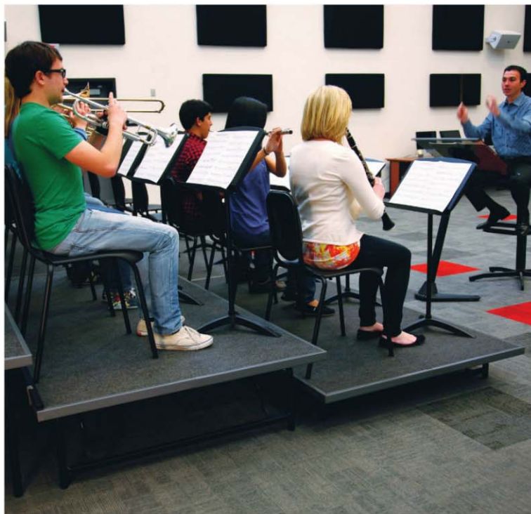
When the space under portable risers is left open, they do not diminish the rehearsal room's overall cubic volume. Portable risers also enable a flat floor for other activities, improving a space's flexibility.
